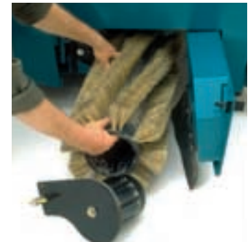
No-tool brush change and no-tool filter change makes maintenance quick and easy.
