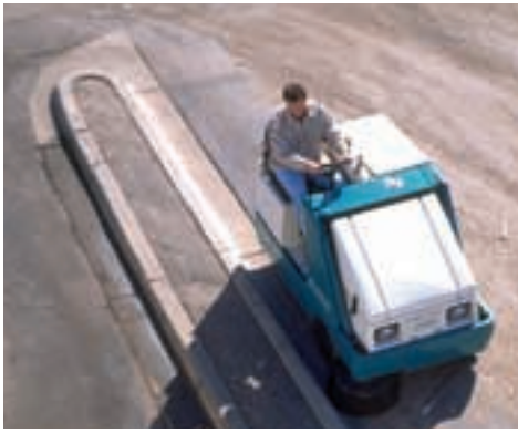
An outdoor package puts pneumatic tires all around for a superior ride on uneven surfaces.
