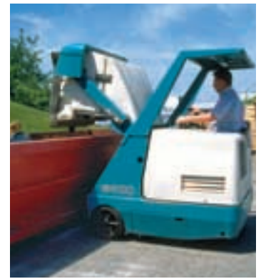
Floating, multi-level dump, non-corrosive hopper, with replaceable steel skidplate, dumps up to 5 ft. (1525 mm) high.
